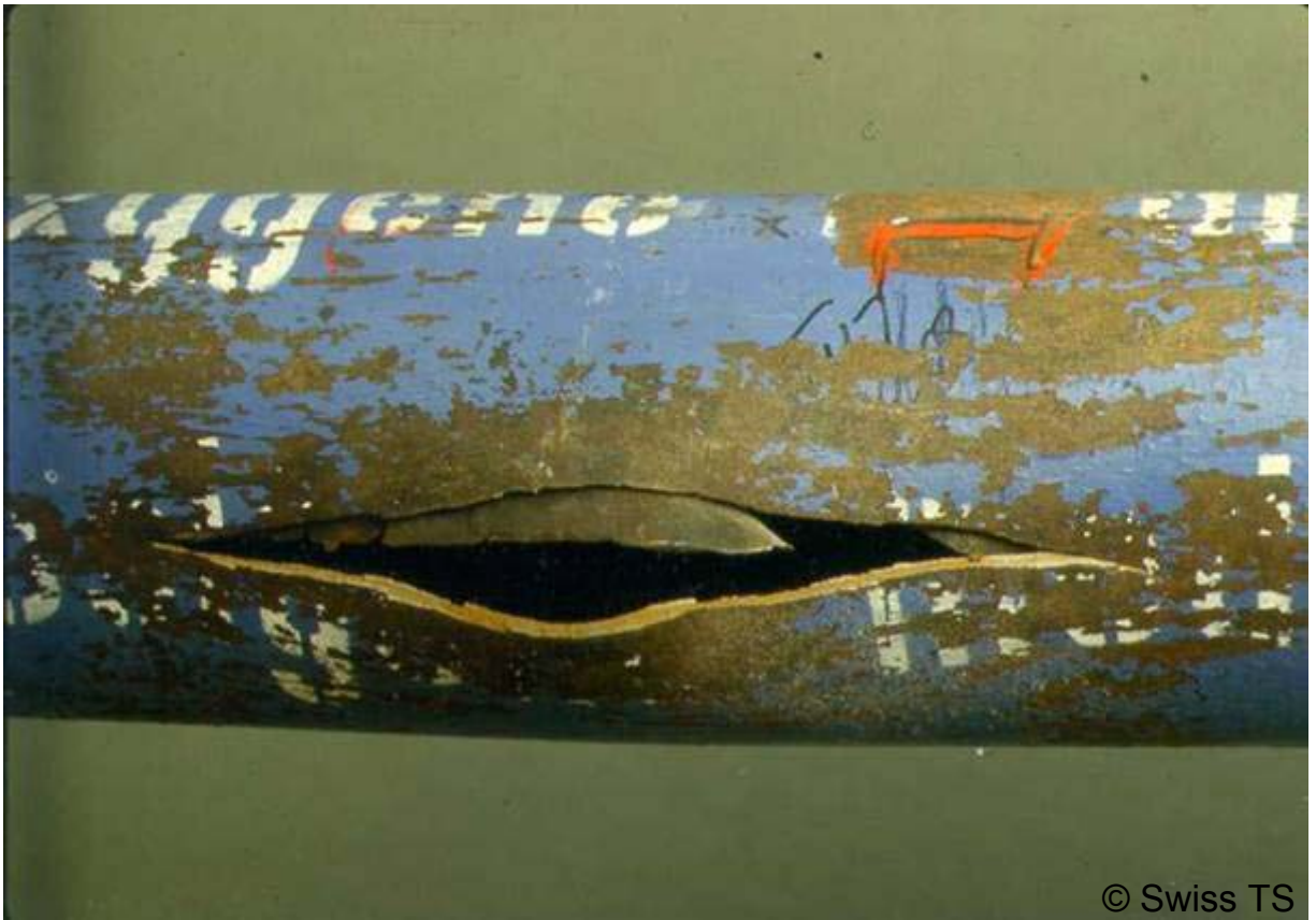
Picture 10: Lamination in the cylindrical part Burst of the cylinder as a result of the flaw and fatigue of material
