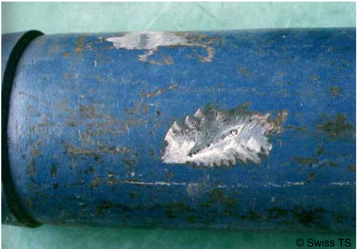
Picture 18: external mechanical damage
