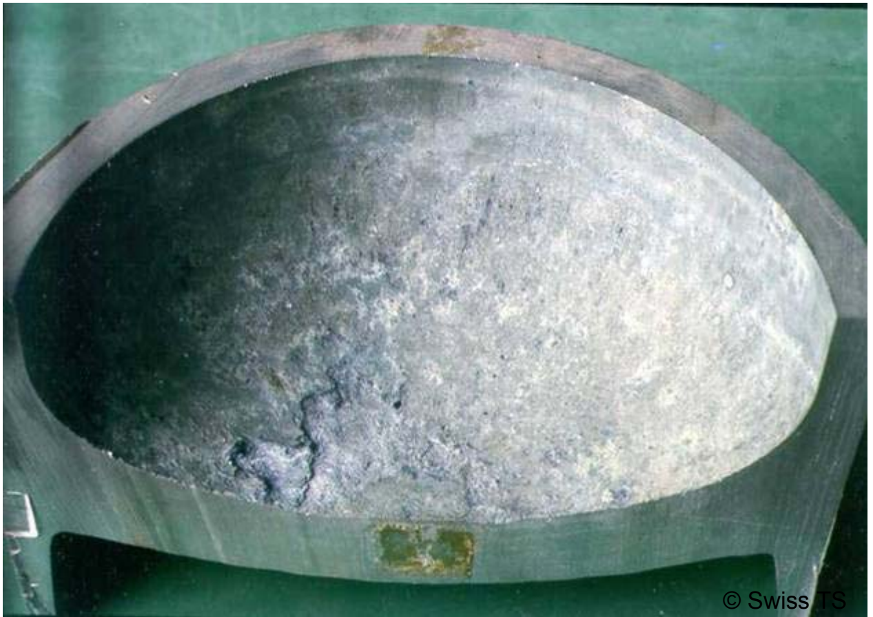
Picture 17: Corrosion of aluminium
