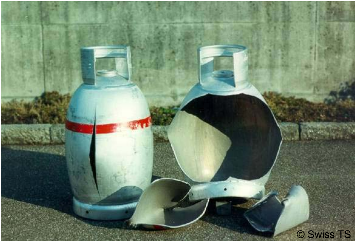
Picture 4: Comparison of water and air pressure burst test
