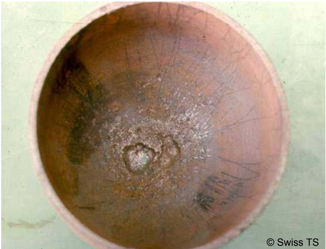
Picture 16: Pitting corrosion
