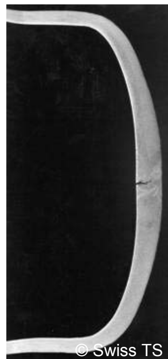
Picture 14 and 15: Inclusion in the base
